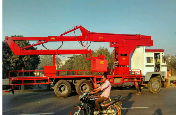
Aerial Work Platform / Truck Crane
