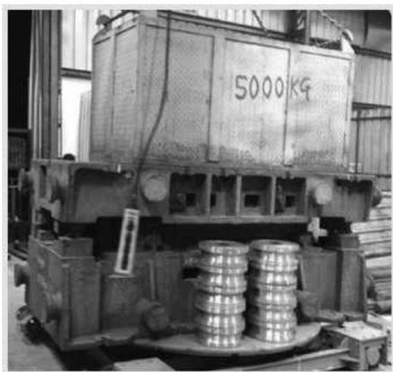
20 Ton Axial load testing for A-30 Bearing
